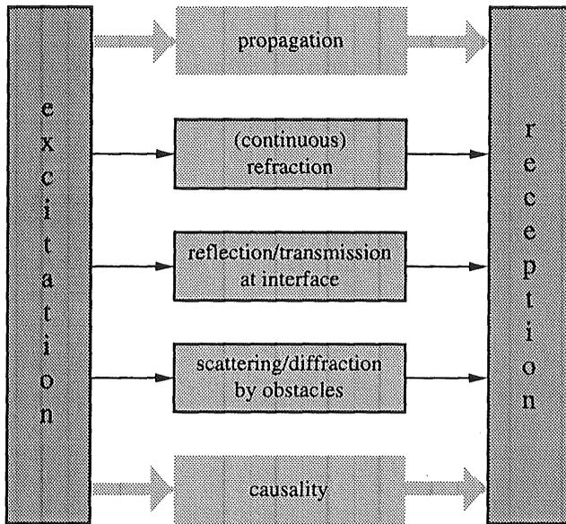
**Figure 17.1** Electromagnetic wave phenomena on their course from source to receiver.
